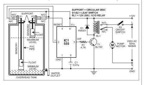
above using an aluminium rod. This arrangement is encased in a PVC pipe and fixed vertically on the inside wall of the water tank. Such sensors are more reliable than induction-type sensors. Sensor 1 senses the minimum water level, while sensor 2 senses the maximum water level (see the figure).
